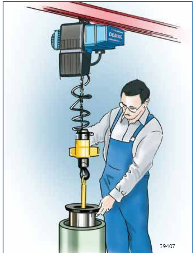
Smooth and precise positioning of a coil in a decoiler
